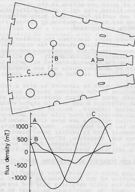
Figure 6 Radial and circumferential flux waves in a core section of a full scale model generator on open circuit
