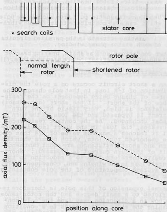
Figure 4 Axial flux density in stator teeth at normal open circuit voltage with normal and shortened rotor lengths
