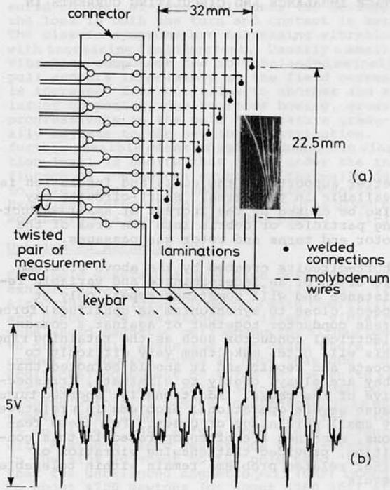
Figure 3 Connections of lamination voltage probes and an example of a 50 Hz interlaminar voltage wave
