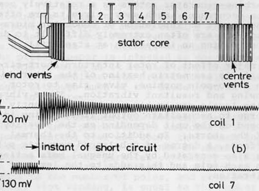
Figure 5 Flux density behind back of core on open circuit and search coil voltages during a sudden short circuit test
