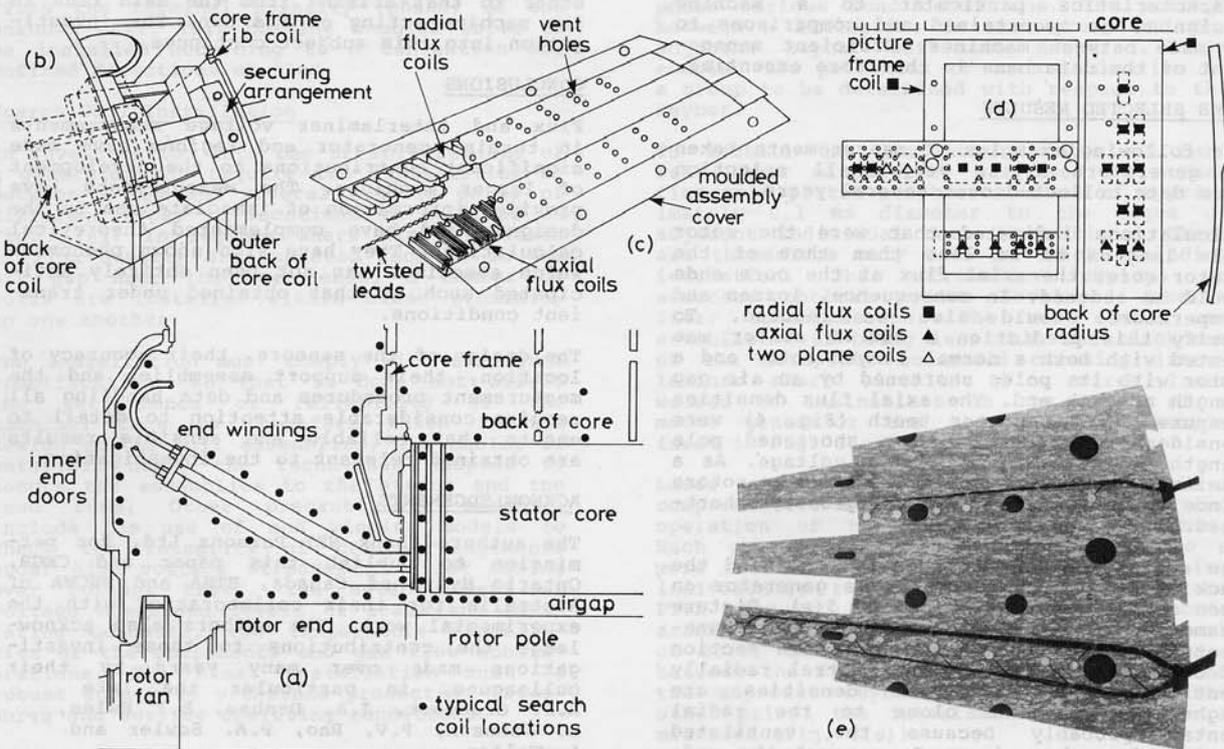
Figure 1 Sectional view of the end region of a generator, typical search coil locations and examples of assemblies
